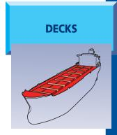
Decks by their very nature are subjected to the most severe operating conditions, regularly awash with seawater, exposed to salt spray, extremes of temperature, impact, mechanical damage and chemical and oil spillage.
