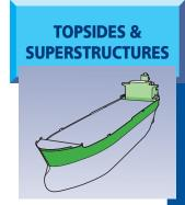
Normally topsides and superstructures are not the areas most exposed to corrosion damage, however, they give a highly visible first impression of the condition of the vessel. To present a favourable impression of the vessel operator it is important to select a system that gives the best combination of anti-corrosive properties together with a durable cosmetic finish.
