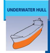
At newbuilding, the selection of the best anticorrosive properties combined with the optimum level of antifouling and foul release systems, is the key to the protection of the underwater hull area. This will ensure long term protection of the vessel and keep maintenance costs to a minimum.
