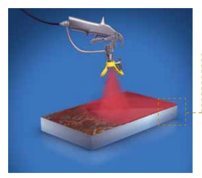
Jotamastic is applied to an aged coating in sound condition prepared to minimum St 2 (or even moist). Waterjetting prepared surfaces with early flash rust are acceptable.
