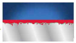
2. Enlarged section through the coated substrate shows Jotamastic penetrating down into the aged sound surface.
